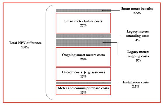
Figure 19: NPV difference between Optimistic and Pessimistic scenarios
