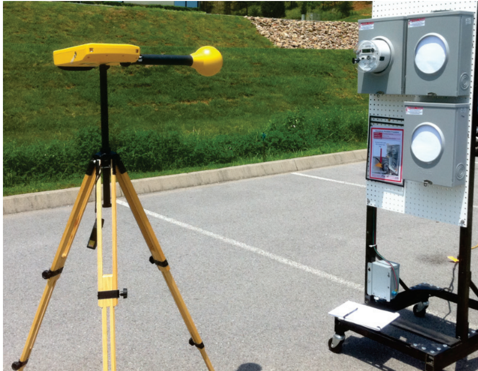
Figure D-4 Measurements with the Silver Spring Meter in open-air test setup.
