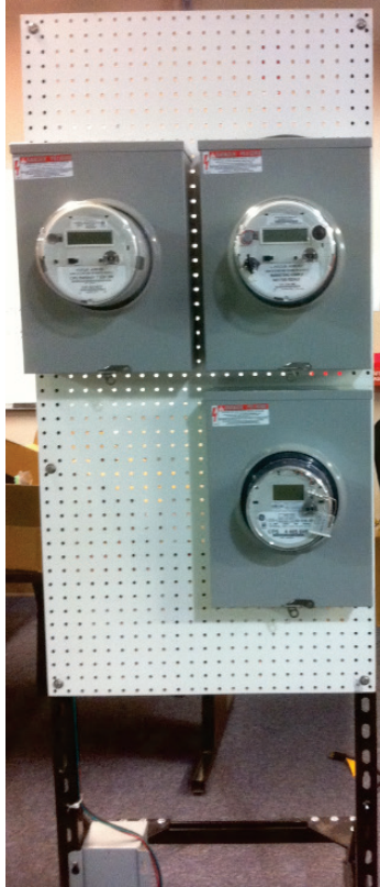
Figure 4-2 Laboratory setup utilized for testing the RF emission from different meter models
