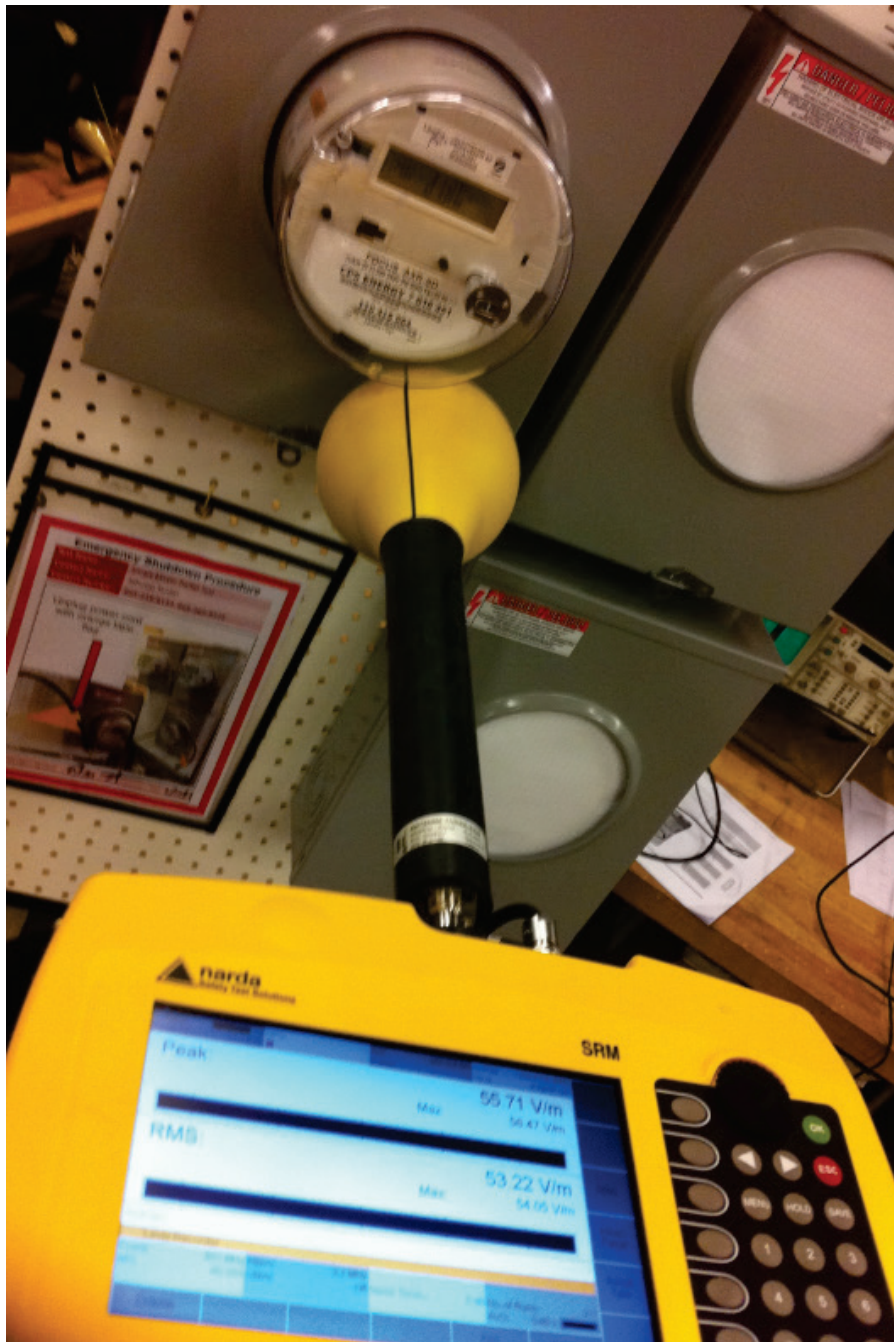
Figure C-5 Maximum detected value of the electric field in the vicinity of the meter.
