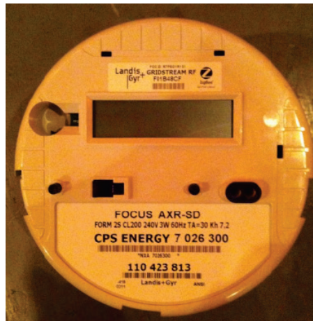
Figure C-1 Landis & Gyr Gridstream meter utilized in the laboratory test
