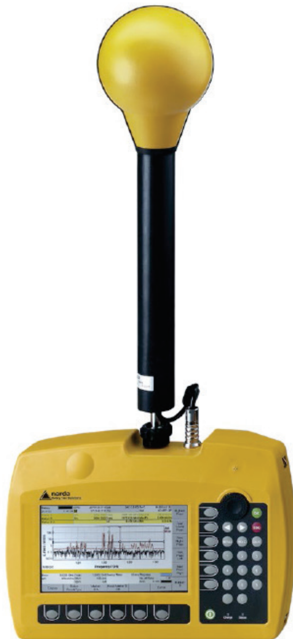
Figure 3-1 NARDA SRM-3006 analyzer utilized for the EM field measurements
