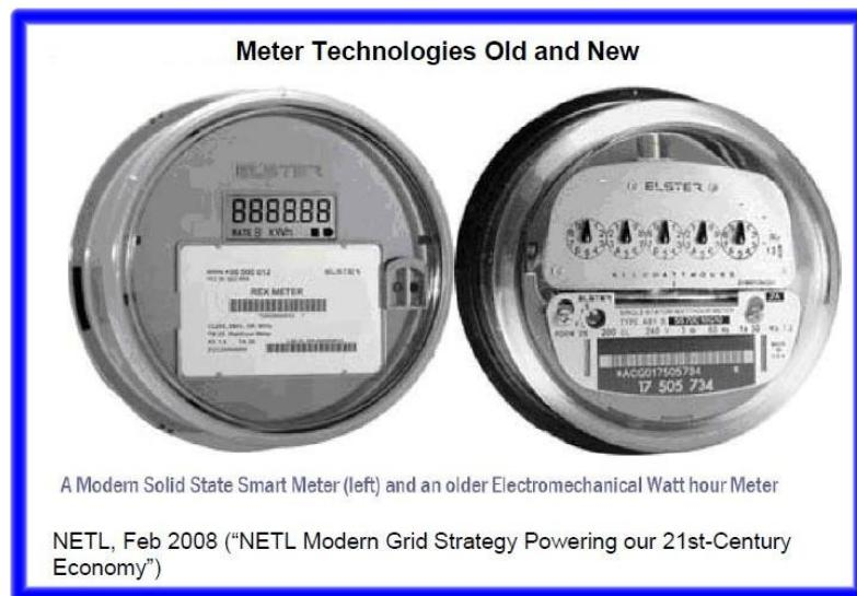
Most new wireless smart meters being installed in the United States and Canada contain two separate transmitters. One transmitter functions within the Neighborhood Area Network (NAN), communicating with the Utility and with other smart meters in the area. The second transmitter exists to function within a Home Area Network (HAN), communicating with “smart” appliances within an individual residence and with an in-home display unit.
