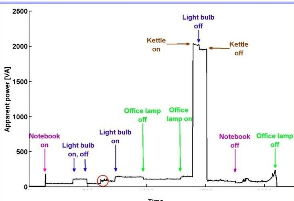
Labeled load curve as output of the AppliSense algorithm
